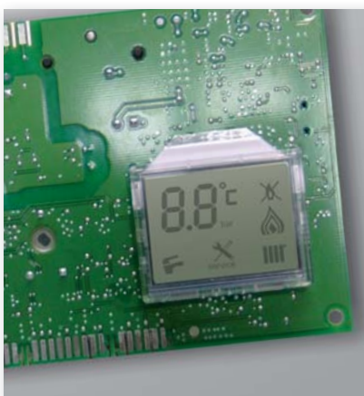
HONEYWELL electronic PCB with microprocessor
